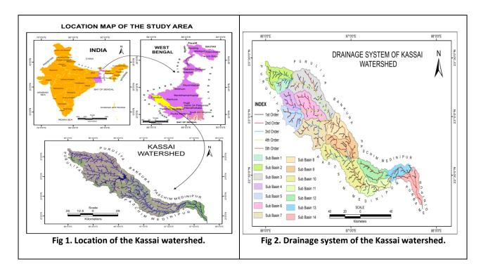
is created for drainage layer of river basin by assigning the attributes. Morphometric analysis is implemented to interpret the watershed characteristics such as linear aspects of the drainage network: stream order, bifurcation ratio, stream length and areal aspects of the drainage basin consists form factor ratio, circularity index, elongation ratio, stream frequency, drainage density and texture ratio of the basin were calculated.
