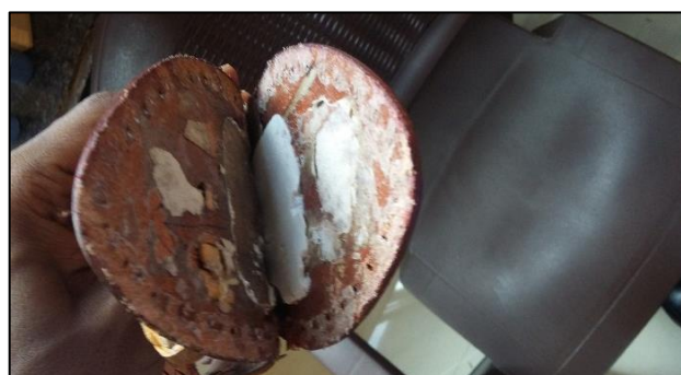
Figure 5. Foam material inserted in two-layer in Kolhapuri crafted footwear
