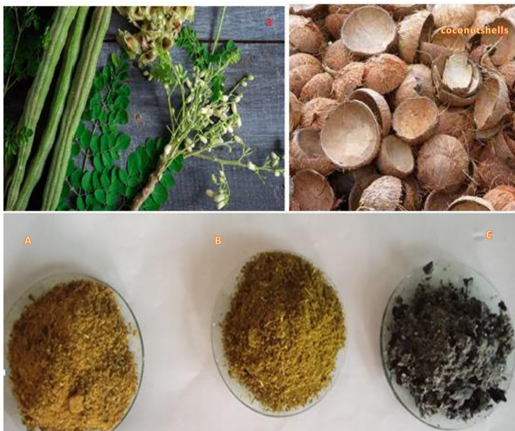
Figure 2. a) Moringa olifera seeds powder b) Moringa olifera leaves powder c) Coconut shells carbon powder.
