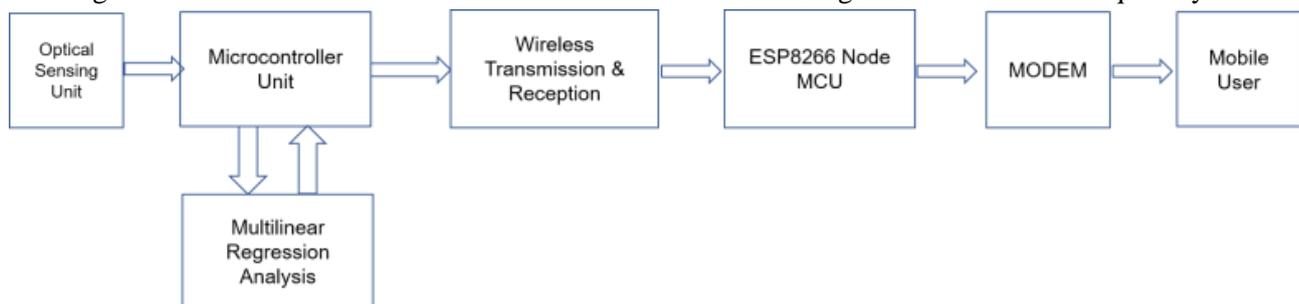
**Figure 1. Block diagram of the developed system**
