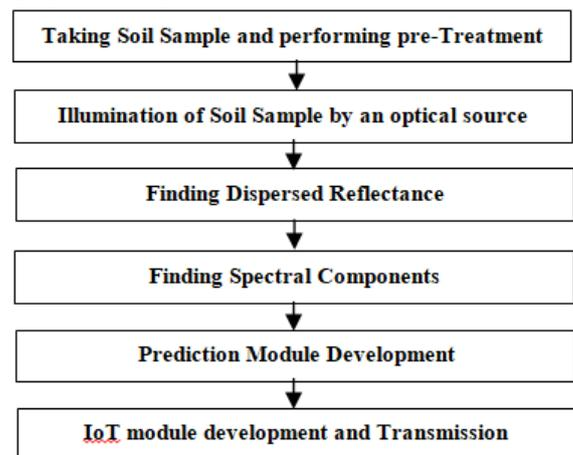
**Figure 2. Steps for Module Design**
