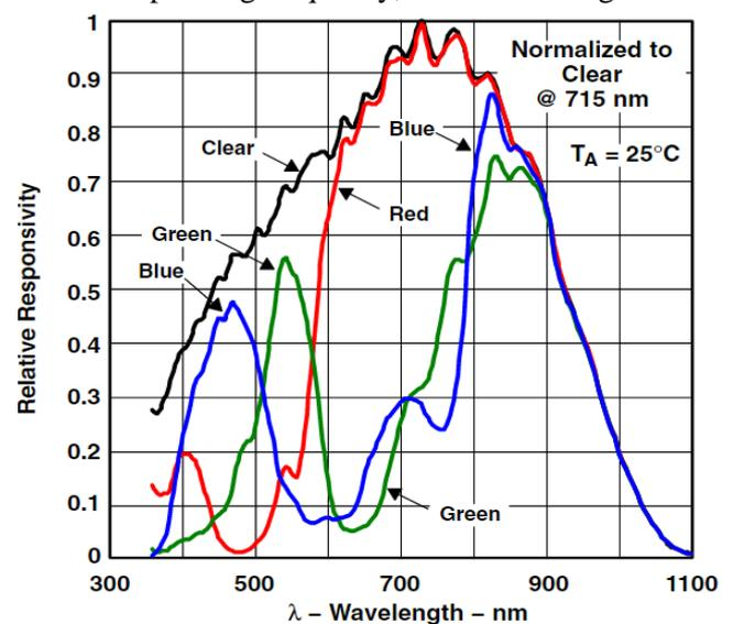
**Figure 4. Photodiode spectral responsivity [TCS3200 Datasheet - Texas Advanced Optoelectronic Solutions]**
