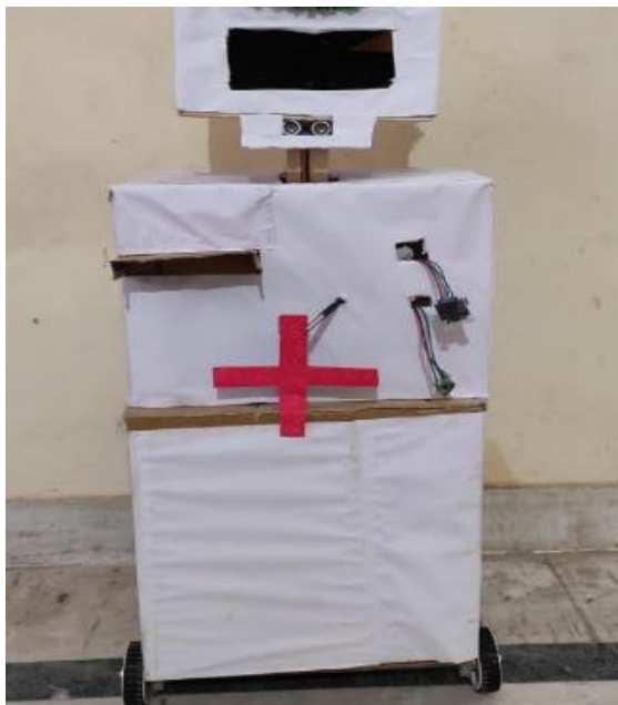
Figure 6. Final prototype Virtual Doctor Robot with display and sensors
