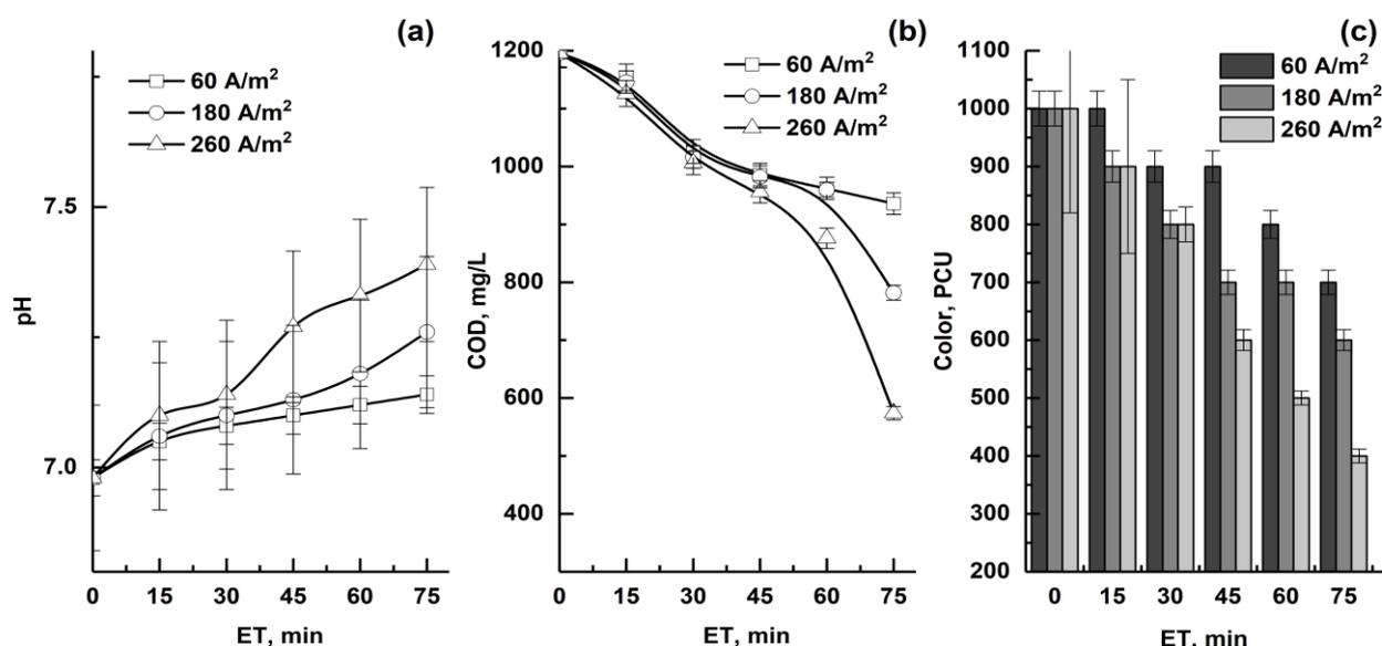
**Figure 2. (a) pH, (b) COD and (c) Colour removal for 4Al electrodes as a function of CDs 60, 180 and 260 A/m<sup>2</sup> up to 75 min ET**
