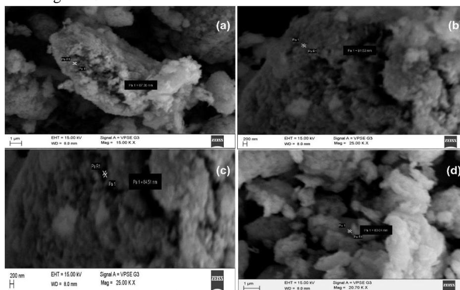
**Figure 3. SEM's Image for  $CuO$ 's Nanoparticle of Leaves Extracts**
