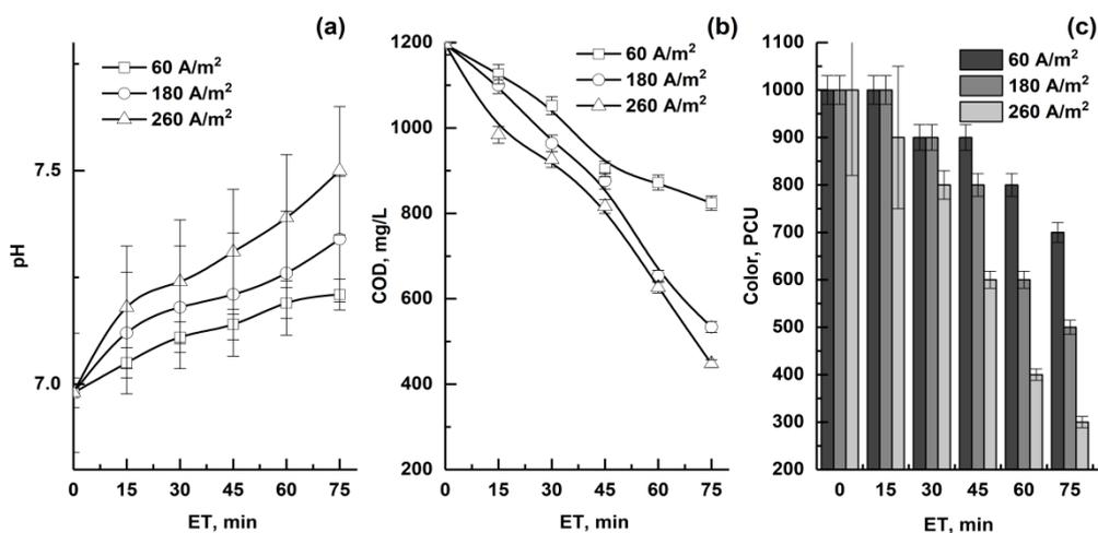
**Figure 1. (A) pH, (B) COD and (C) Colour Removal using 4SS Electrodes as A Function of CDs 60 – 260 A/M2 Up To 75 Min ET**
