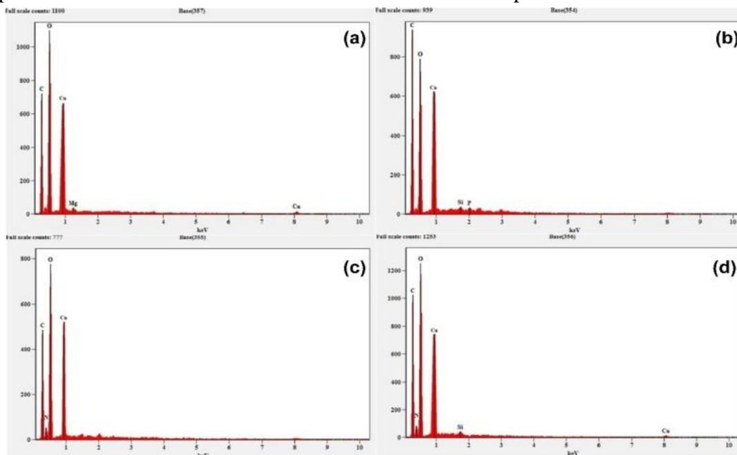
**Figure 4. EDAX Image for CuO's Nanoparticle Synthesized by Utilizing Leaves Extracts**
