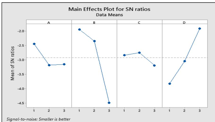
Figure 2. Ra's S/N ratio plot.
