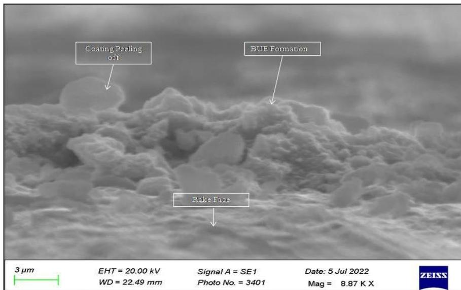
Figure 5. SEM image of tool insert TiAlN.
