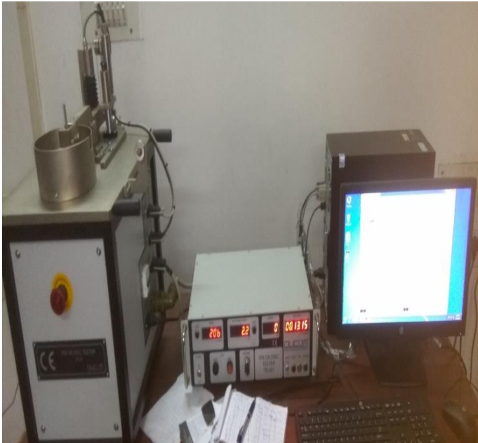
Figure 2. (A) & (B) Wear test sample dimension and (C) Pin-on-Disc wear test Machine.
