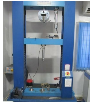
Figure 7. Universal testing machine
