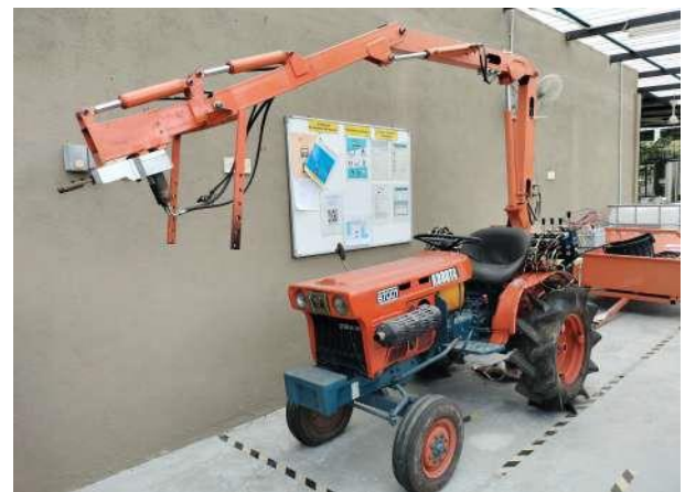
Figure 3. Available excavator with boom and arm mounted on a tractor (model B7001 from Kubota company)
