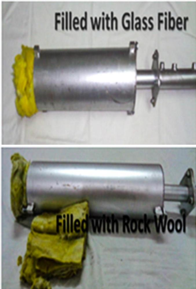
**Figure 9. Sound-absorbing materials were used during validation.**
