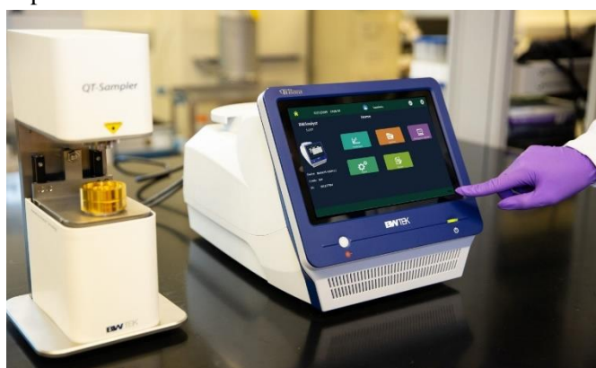
Figure 3. QTRam instrument used for Raman Spectroscopy analysis
