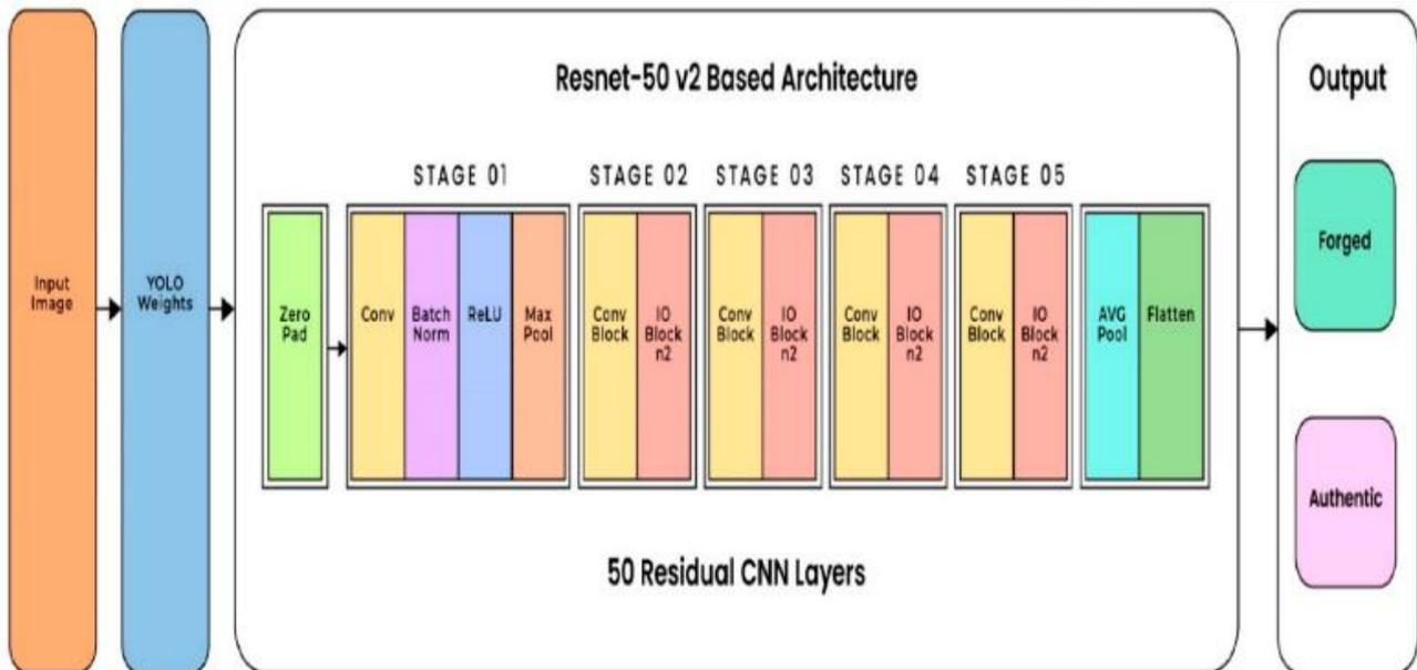
Figure 4. ResNet50 V2 Architecture [Source: Adapted from Qazi et al. (2022)].
