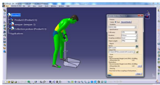
Figure 10(i). Lifting result when time per lift is 120 seconds for lifting 20 kg weight
