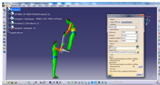
Figure 12(i). Lifting result of external laborer when time per lift is 120 seconds for lifting 20 kg weight
