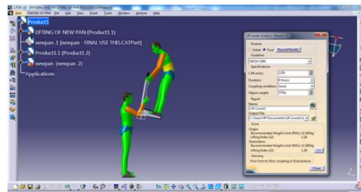
Figure 12(ii). Lifting result of external laborer when time per lift is 120 seconds for lifting 15 kg weight
