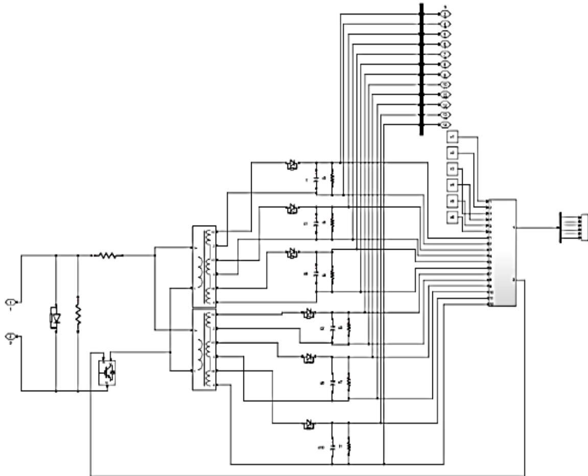
**Figure 4. DC-DC Flyback converter with Multi-Output.**
