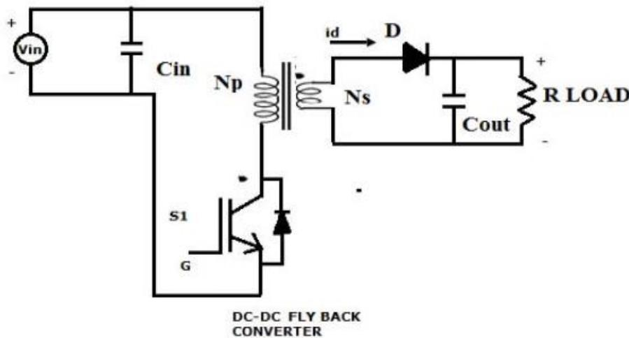
Figure 3. DC-DC Flyback Converter.
