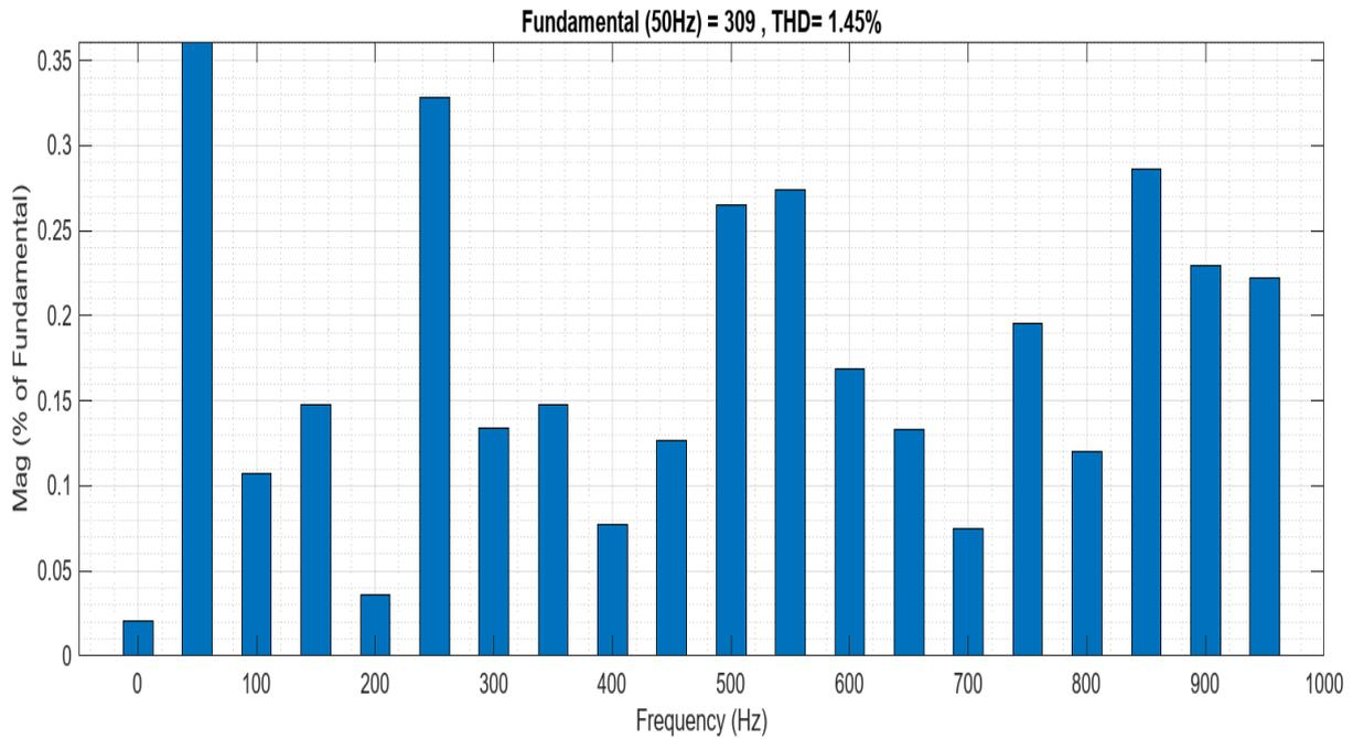
**Figure 14. Harmonic analysis of proposed Dstatcom Model.**
