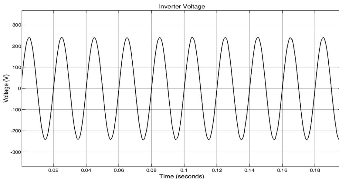
**Figure 5. Proposed Inverter Output.**
