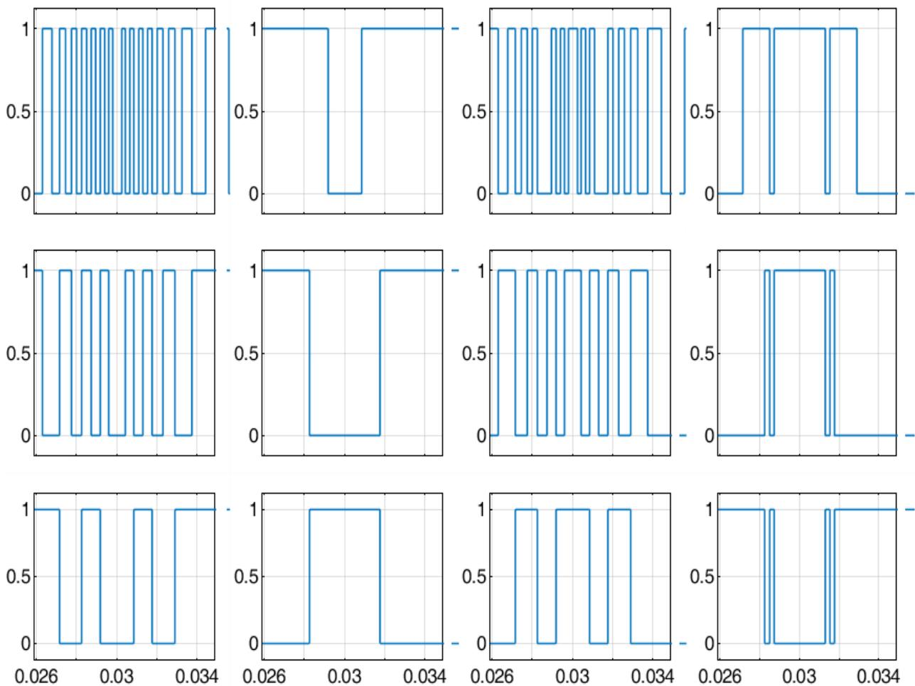
Figure 12. Gate Pulses to Inverter.
