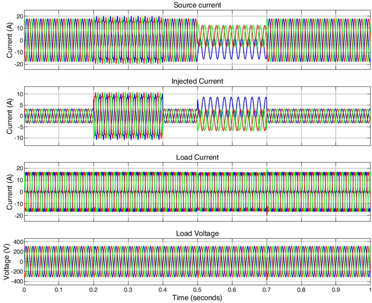
**Figure 13. Source current, compensated current, load current and load Voltage.**
