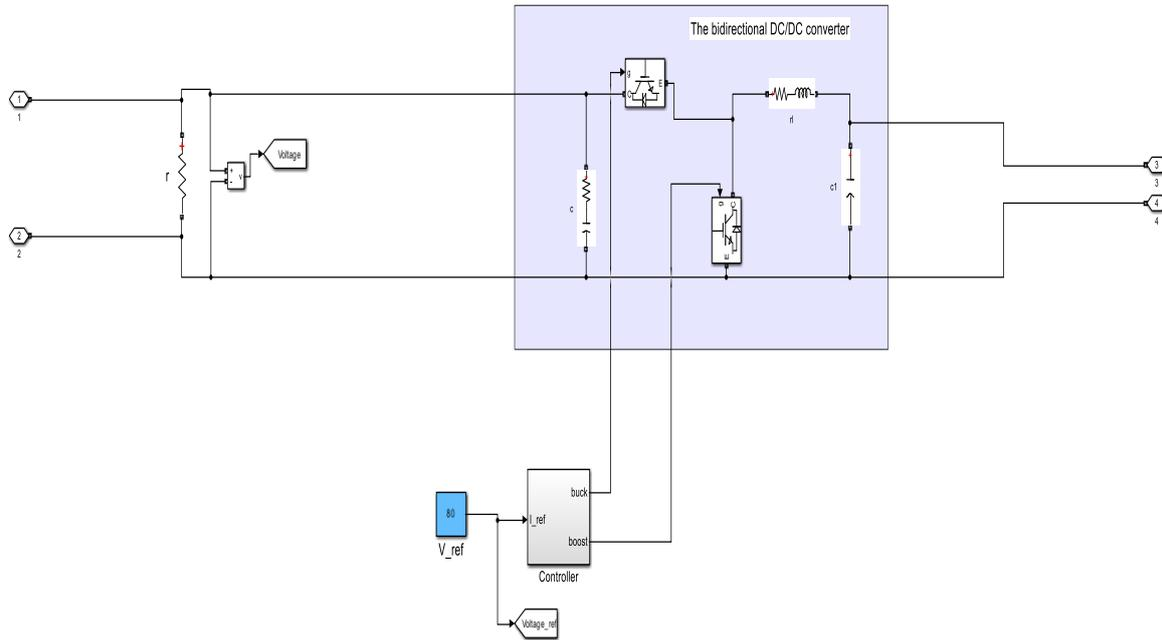
Figure 2. Bidirectional DC-DC Converter.
