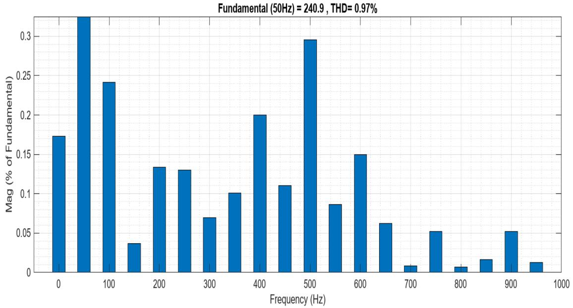
Figure 11. Harmonic analysis of the proposed inverter.
