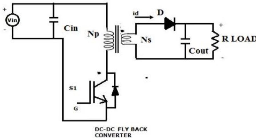
Figure 3. DC-DC Flyback Converter.
