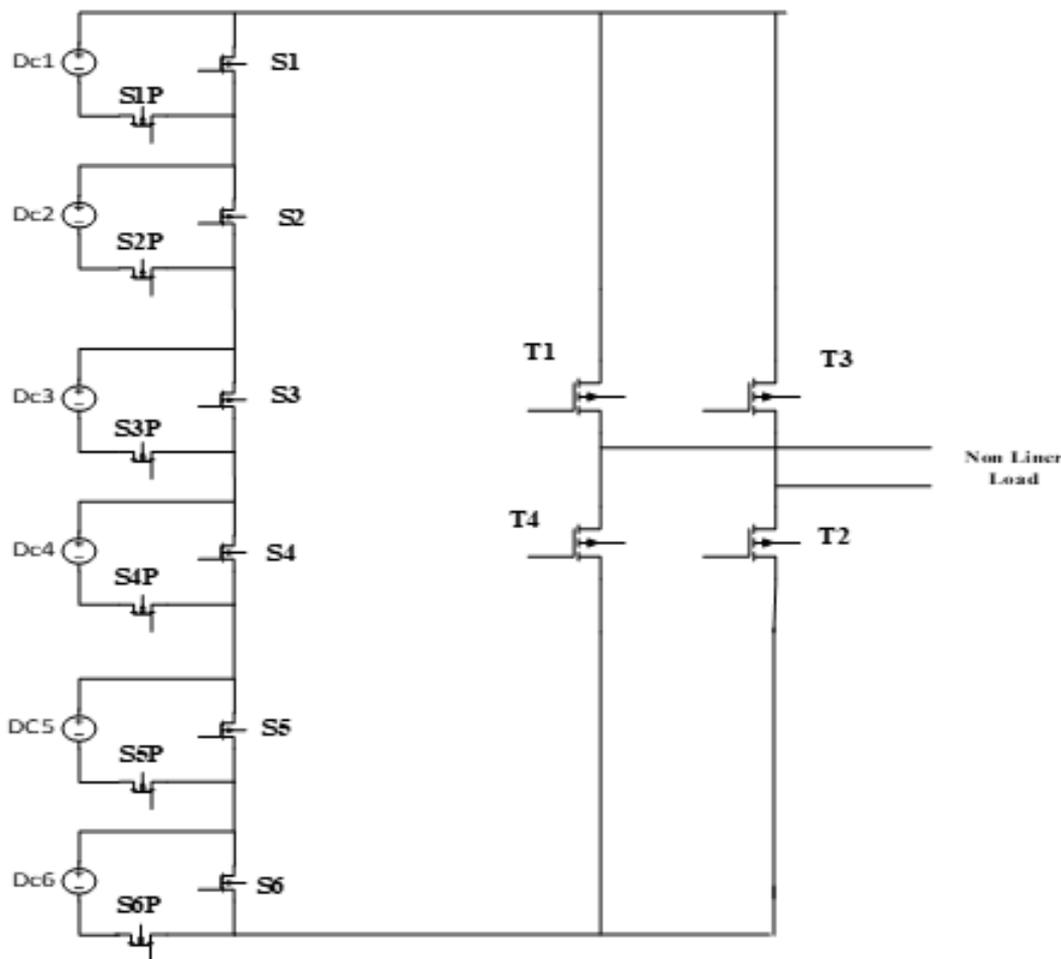
**Figure 1. Proposed 125-level MLDCL Inverter**
