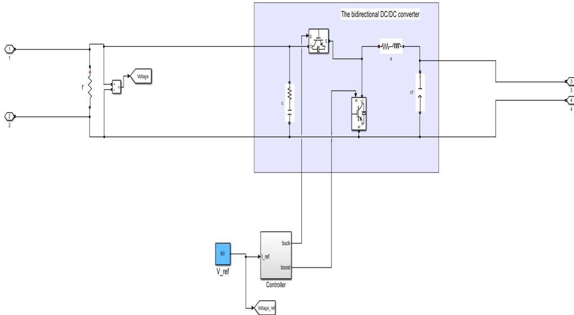
Figure 2. Bidirectional DC-DC Converter.
