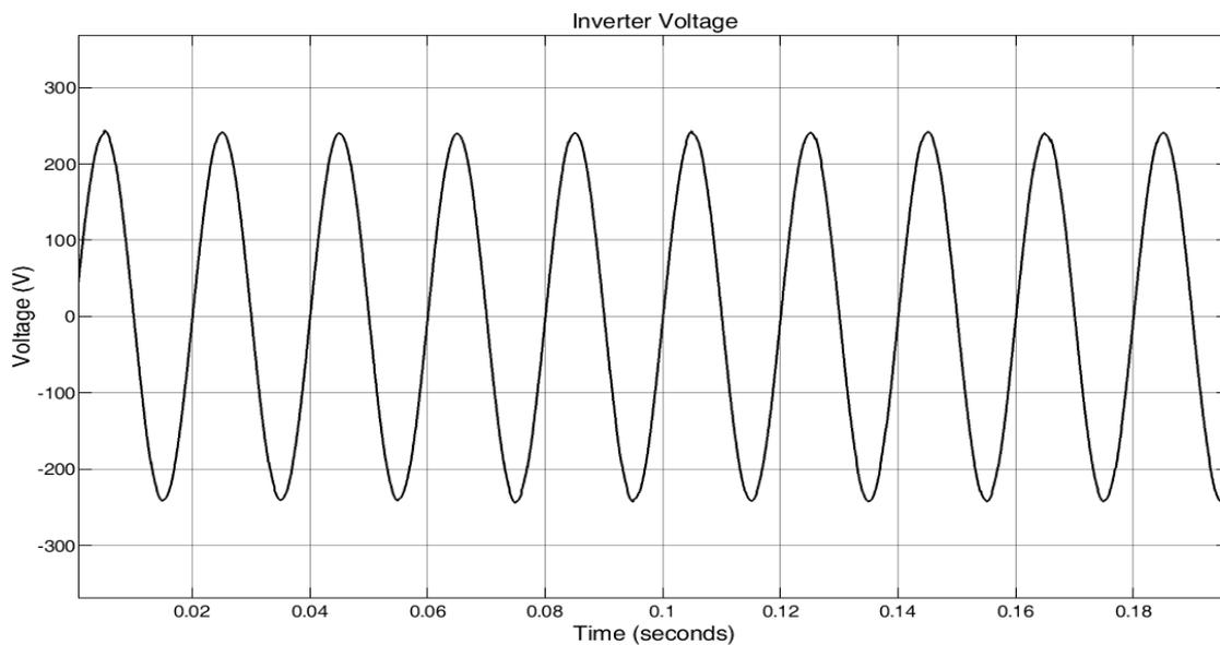
**Figure 5. Proposed Inverter Output.**
