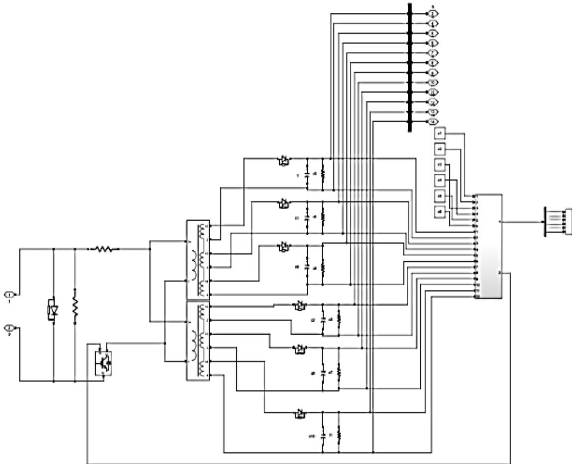
**Figure 4. DC-DC Flyback converter with Multi-Output.**
