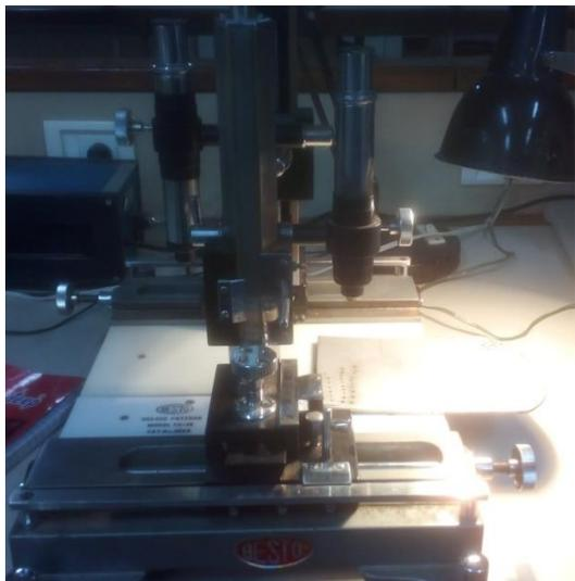
Figure 4. Traveling Microscope
