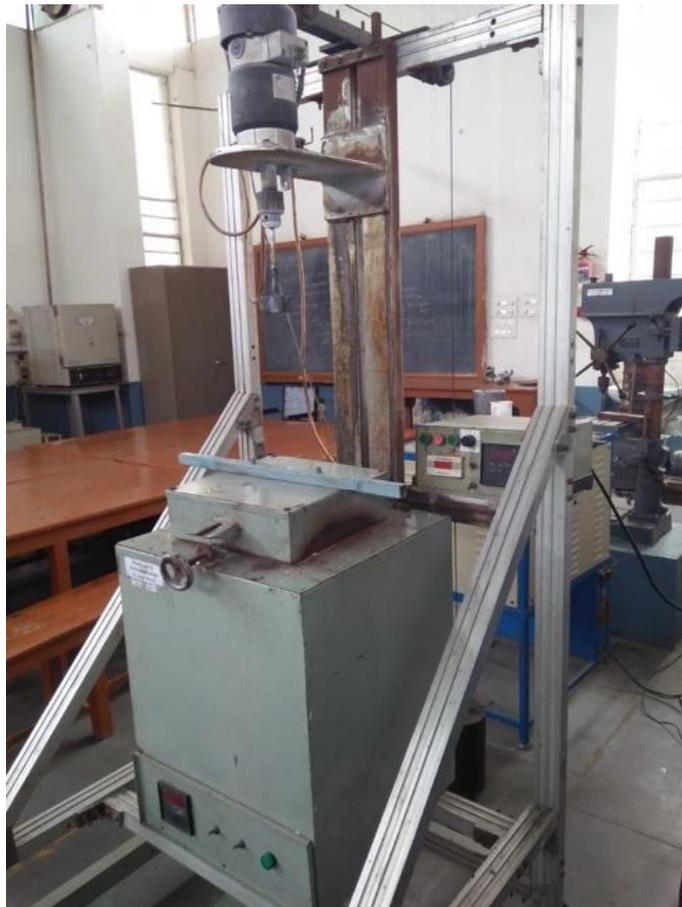
**Figure 2. Stir casting setup.**
