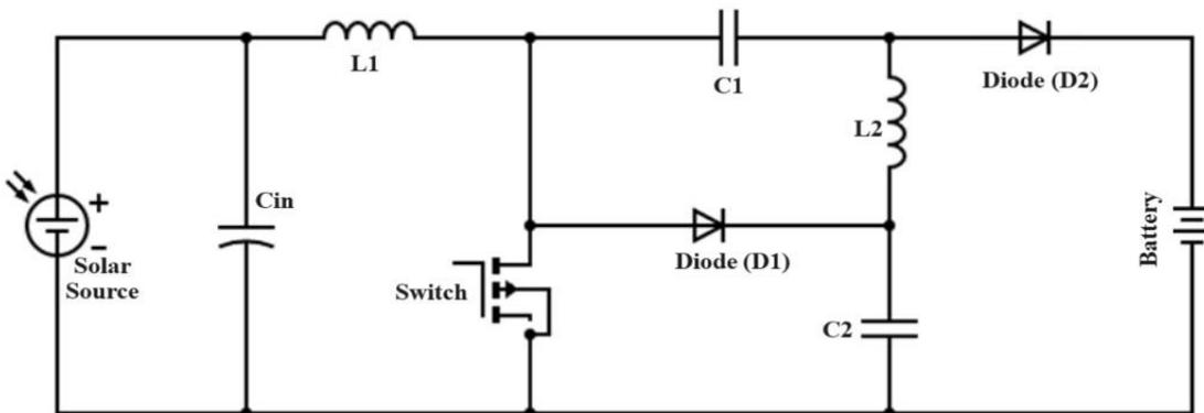
**Figure 4. Schematic of the modified SEPIC converter**
