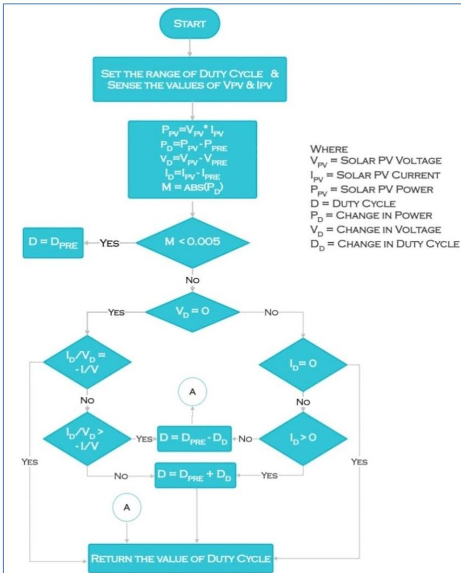
Figure 2. Flowchart for Incremental Conductance MPPT.
