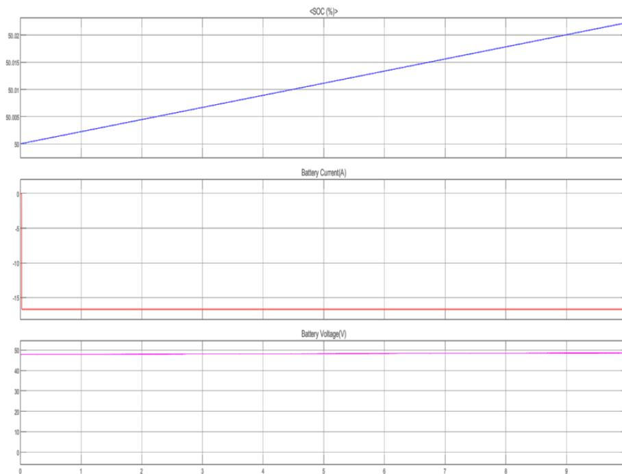
Figure 7. Battery charging results for the modified SEPIC converter without MPPT.
