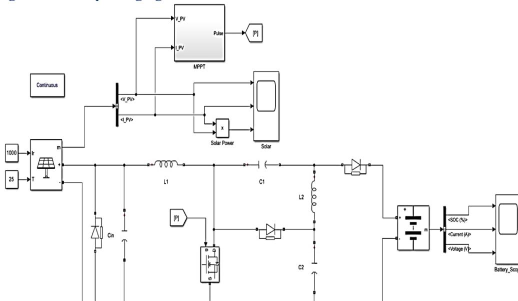
Figure 8. MATLAB/Simulink model of the modified SEPIC converter with P&O MPPT.
