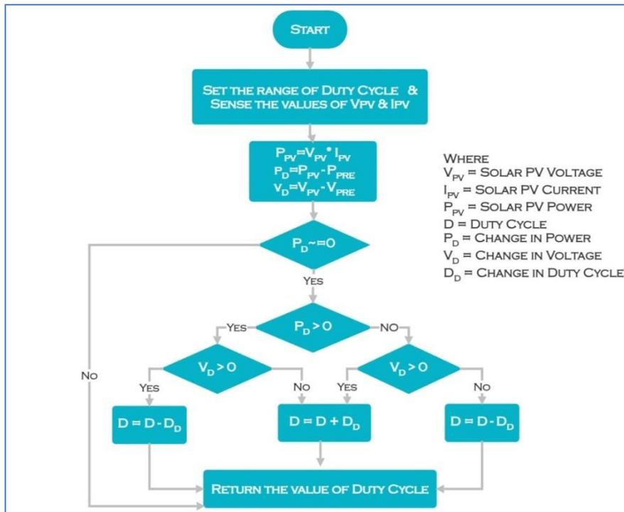
Figure 1. Flowchart for Perturb & Observe MPPT.
