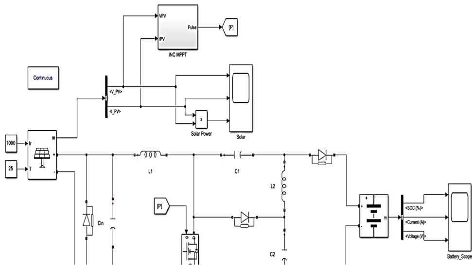
Figure 11. MATLAB/Simulink Model of the modified SEPIC converter with INC MPPT.
