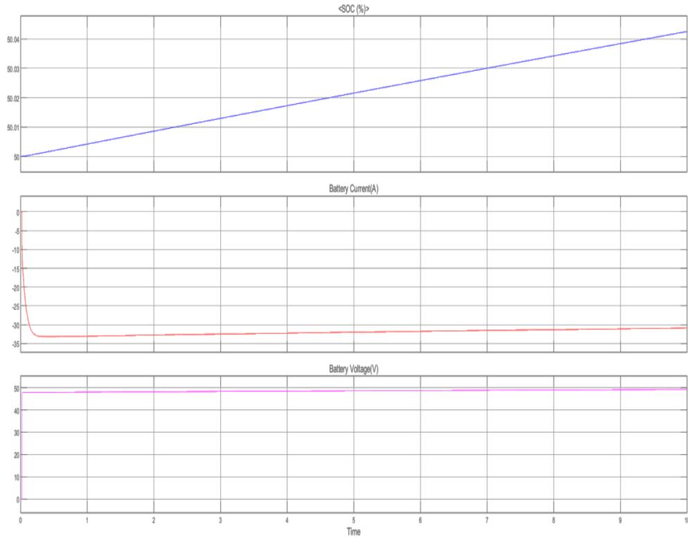
Figure 13. Battery charging results for the modified SEPIC converter with INC MPPT.
