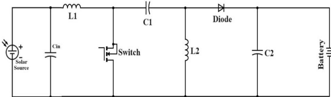
**Figure 3. Schematic of the traditional SEPIC converter.**
