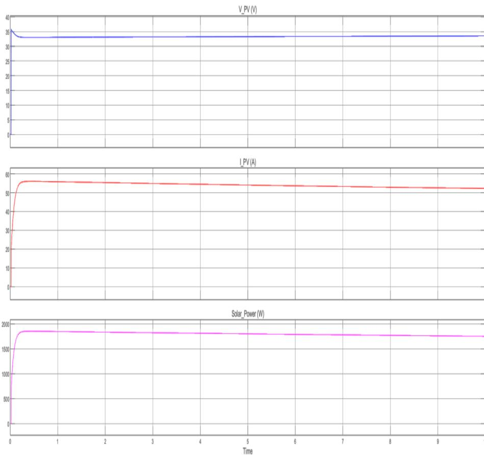
Figure 12. PV characteristics results of the modified SEPIC converter with INC MPPT.
