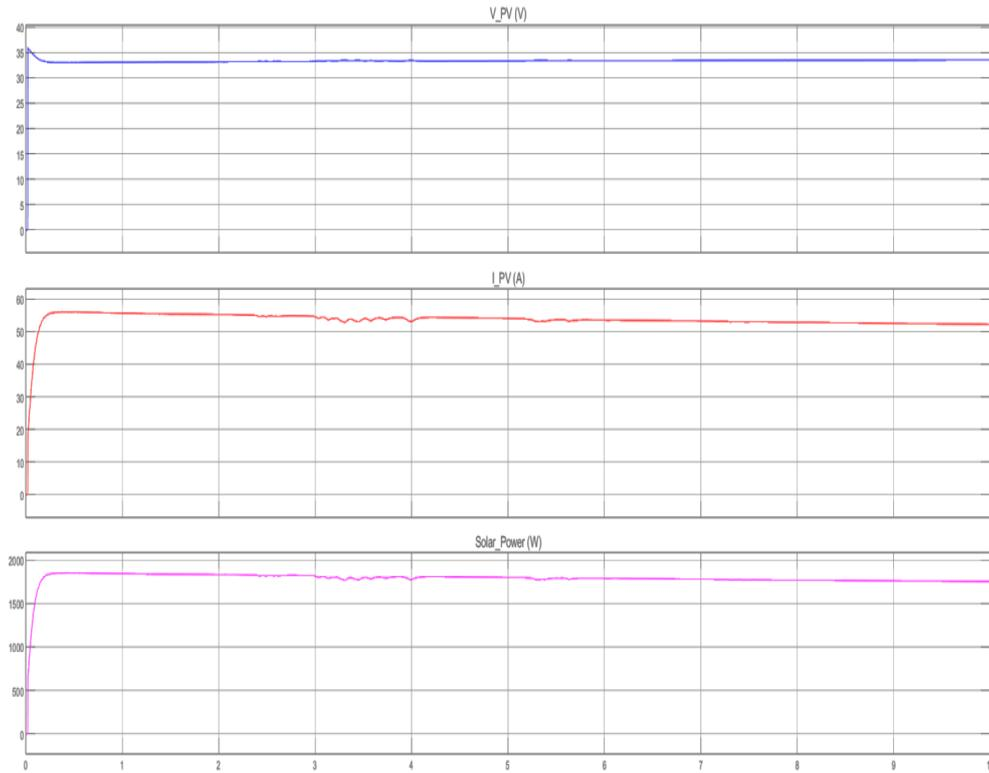
Figure 9. PV characteristics results for the modified SEPIC converter with P&O MPPT.
