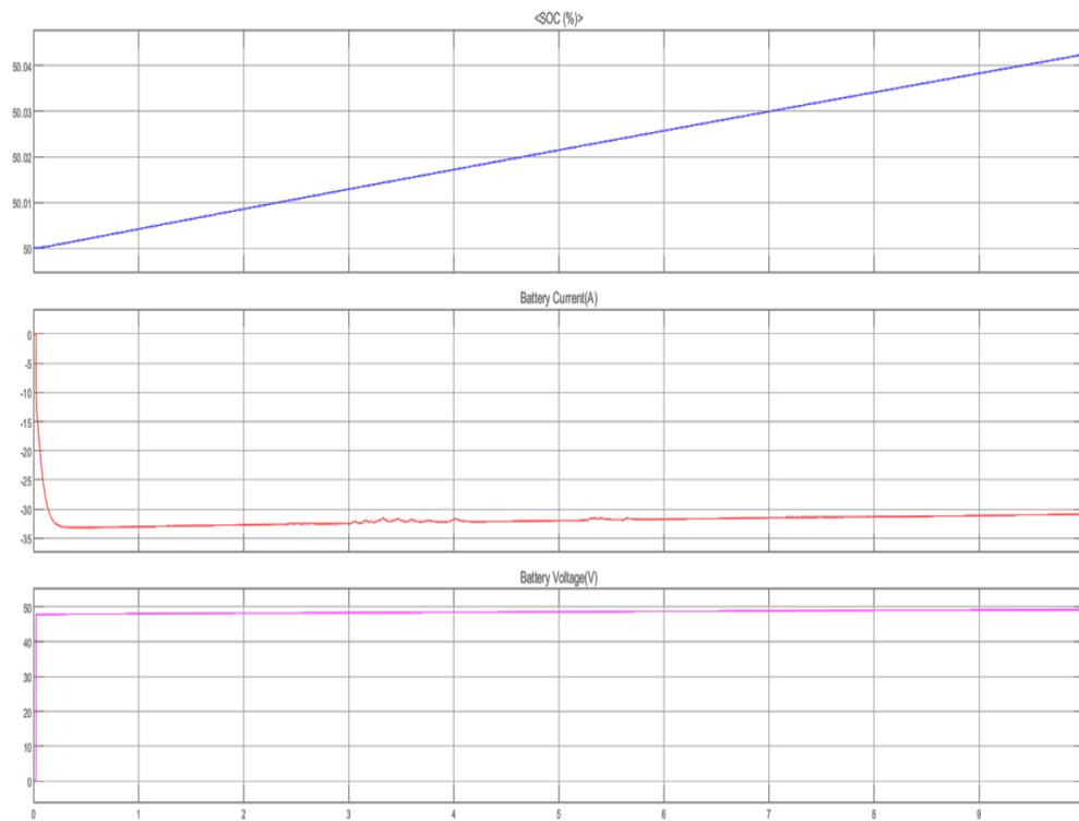
Figure 10. Battery charging results for the modified SEPIC converter with P&O MPPT.
