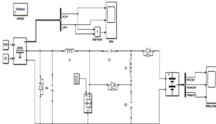
**Figure 5. MATLAB/Simulink Model of the modified SEPIC converter without MPPT.**
