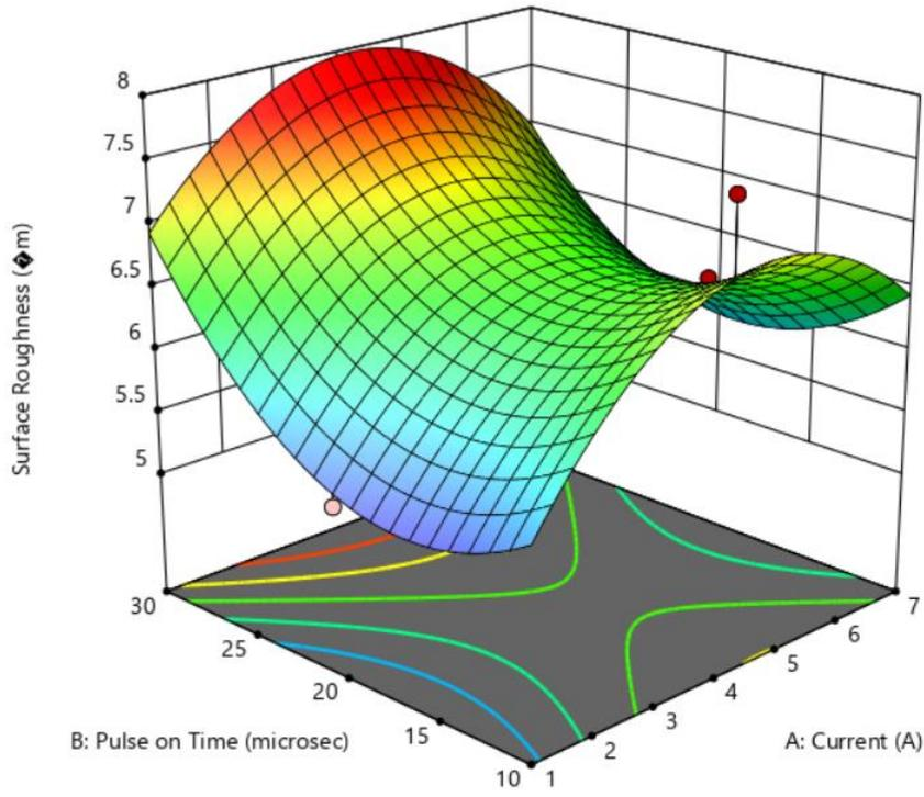
**Figure 3. Surface Plot for Surface Roughness with pulse on time and current.**
