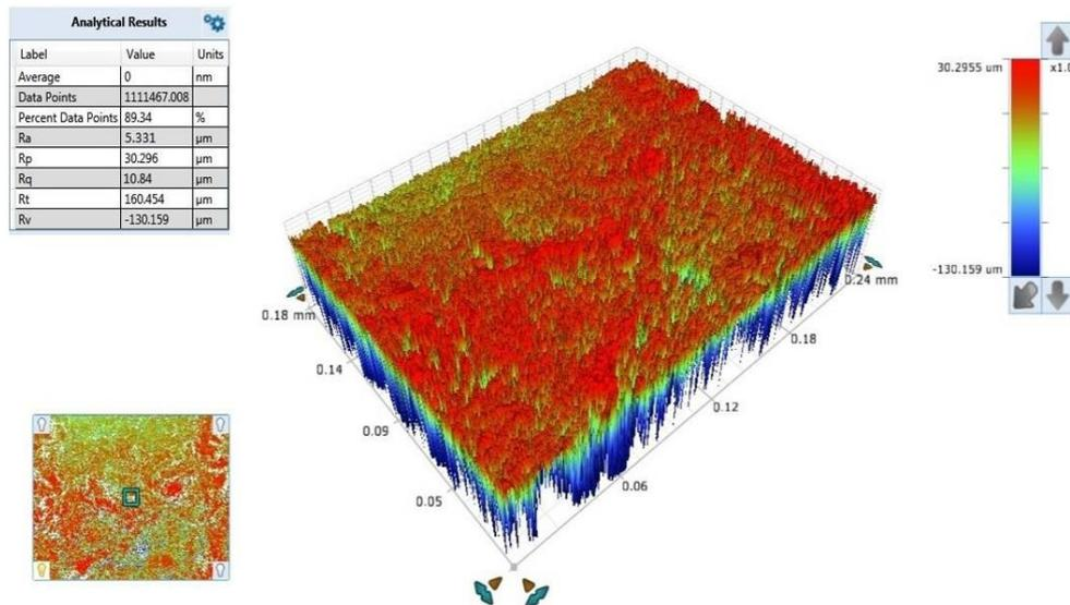
**Figure 2. Surface Roughness measurement of Sample 4 using white light interferometry.**
