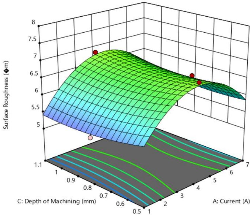
**Figure 4. Surface Plot for Surface Roughness with current and depth of machining.**
