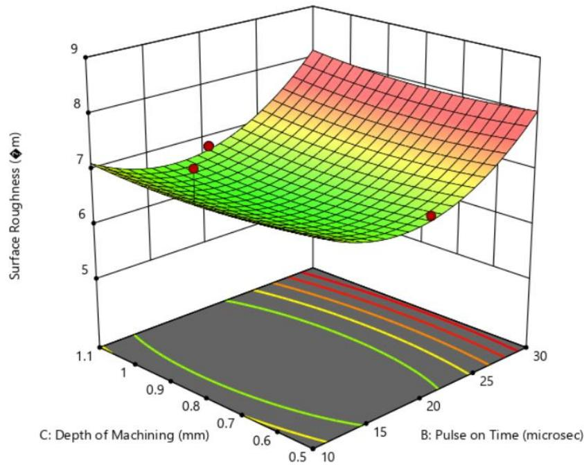
**Figure 5. Surface Plot for Surface Roughness with depth of machining and pulse on time.**
