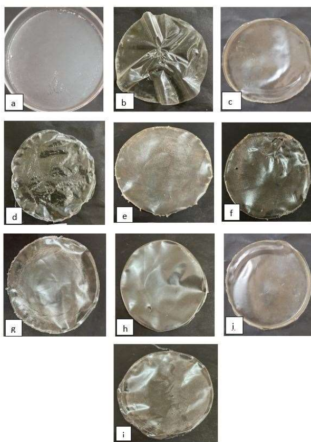
Figure 1. Composite Biopolymer films. a- sample 1, b- sample 2, c- sample 3, d- sample 4, e- sample 5, f- sample 6, g- sample 7, h- sample 8, i- sample 9, j- sample 10 showing outcome of the films with different percentage of gelatin and polyvinyl alcohol out of many trials.
