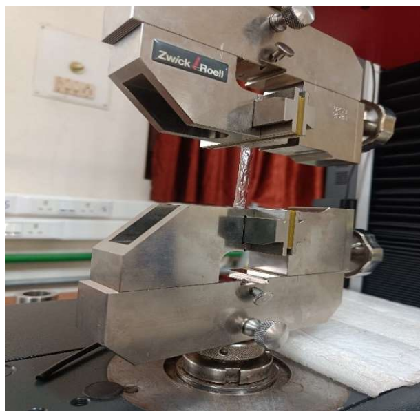
Figure 3. Tensile strength Determination of tensile strength of the biopolymer film with Zwick/Roell instrument showing stretching of the film. 56.6±3.13 of sample 9 is the highest tensile strength observed rather than other samples.
