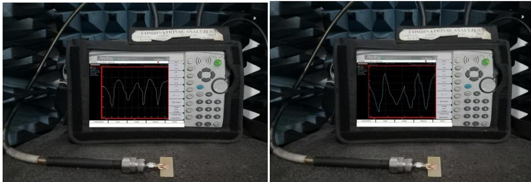
Figure 19. Spectrum Analyzer output of Two-layer Antenna (a) Return loss from 25 GHz to 45 GHz (b) VSWR from 25 GHz to 45 GHz.
