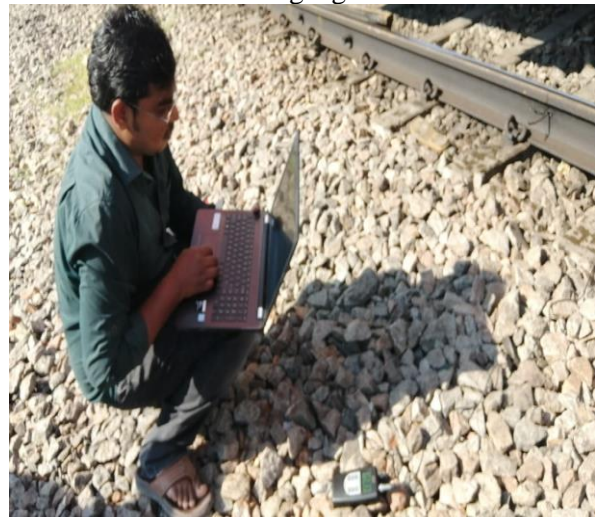
d) Testing the rubber pads placed under the rail track with vibro-meter.
