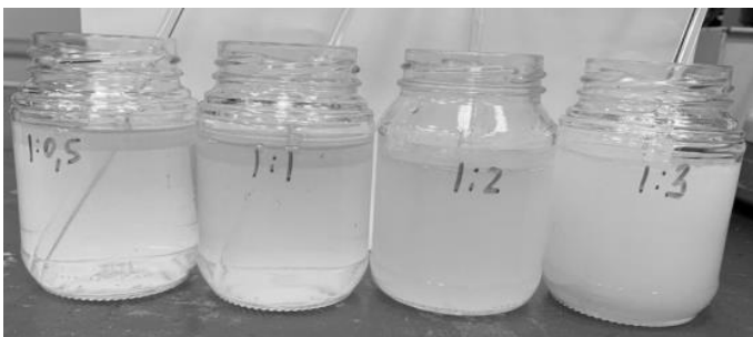
Mixing at 400 rpm for 10 min and ultrasonic treatment at a frequency of 22 kHz and 100% power for 5 min
