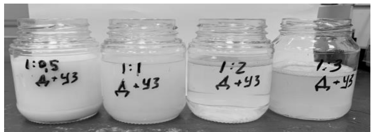
Dispersion at 17,500 rpm for 5 min and ultrasonic treatment at a frequency of 22 kHz and 100% power for 5 min
