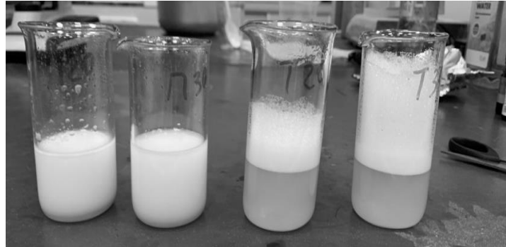
Figure 3. Emulsion samples with emulsifier concentration of 20% and 30% after ultrasonic treatment: from left to right - PEG 20%, PEG 30%, TWEEN 80 20%, TWEEN 80 30%.
