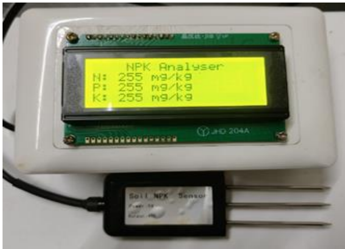
Figure 2. Ground N-P-K sensors with display.
