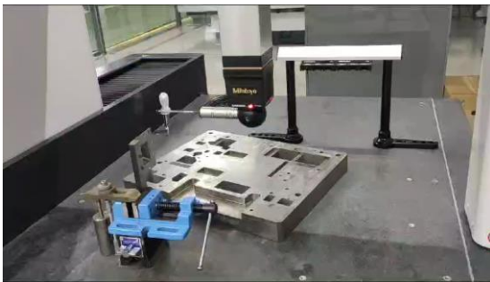
Figure 6. (a). 'Mitutoyo' CRYSTA-Apex S 9108; (b) Measurement of formed component profile.
