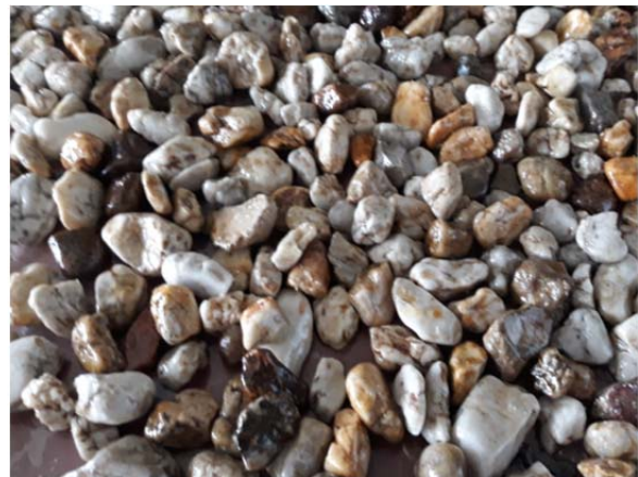
Fig. 3. Epoxy resin coated aggregates
