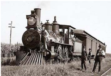
Fig. 4 Sierra Railway #3 was built in 1891 and has a top speed of about 50 MPH [6]
