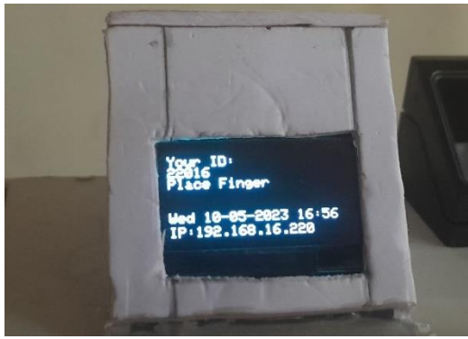
Figure 4.2.2 Registration Proceeding on Hardware
