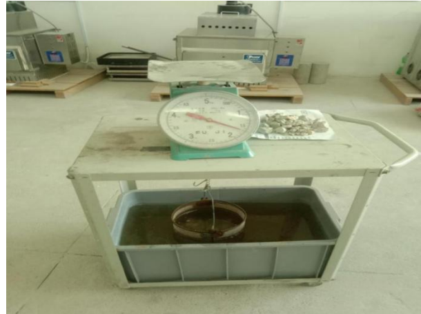
Fig. 4: Water Absorption & Specific Gravity test Setup
