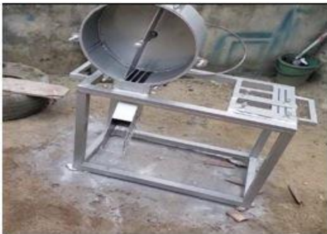
(a) Cracking drum on main frame
