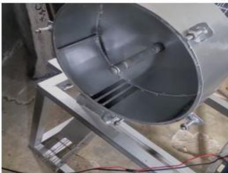
(c) Cracking hammer shaft
