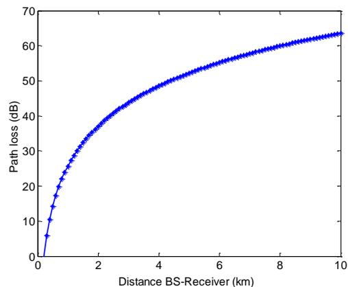
**Fig. 4. Path loss due to log-normal shadowing using Walfish-Ikegami model**
