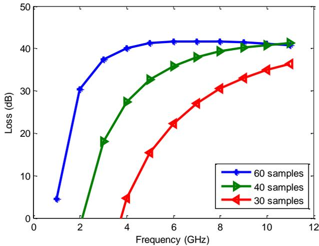
**Fig. 2. Diffraction loss due to single-rounded obstacle**
