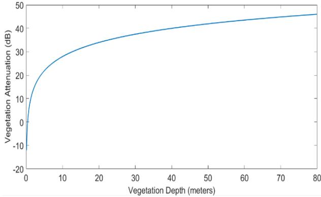
**Fig. 3. Loss due to vegetation using ITU-R model at 11 GHz**
