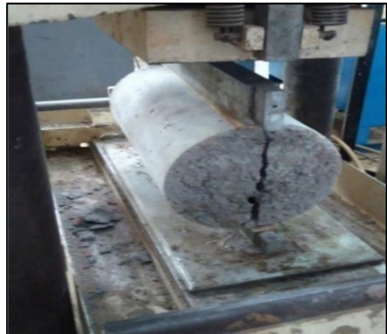
Figure 5. Testing of tensile strength samples (a) Sample of loaded specimen; (b) Sample of failed specimen
