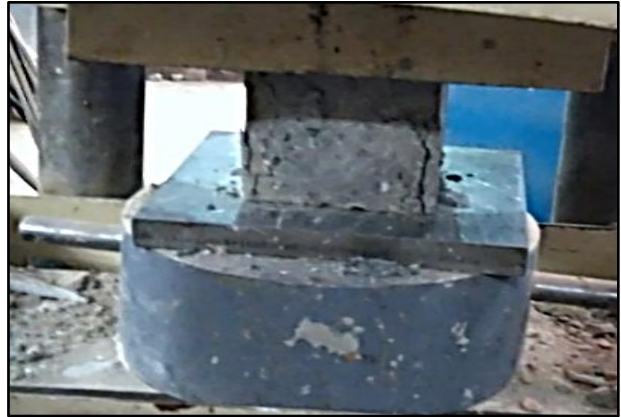
Figure 4. Failed compressive strength sample
