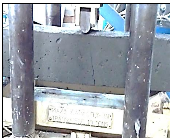
Figure 6. Testing of flexural strength samples (a) Loaded sample; (b) Failed sample
