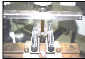
Figure 3: Flexural strength testing of PMMA specimen by four-point bend test
