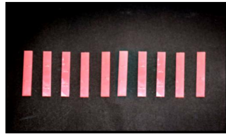
Figure 1: PMMA specimen milled to desired ISO Dimension
