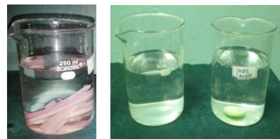
Figure 3a: Distilled water immersion to remove residual monomer. Figure 3b. Control (distilled water) and Experimental immersion (denture cleanser)
