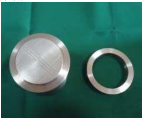
Figure 1: stainless steel master die –metal base with `detachable cylindrical ring
