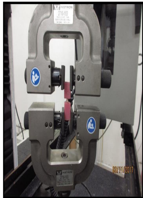
FIG:1-TESTING OF MICROTENSILE BOND STRENGTH
