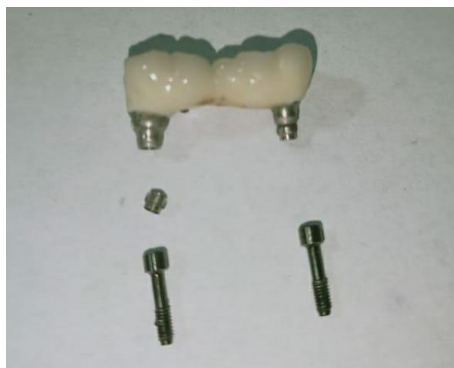
Figure 1: Fracture at the abutment internal helix
