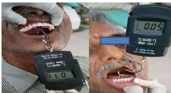
Figure 10: Retention assessment with forcemeter
