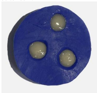
Fig 1. Composite disc preparation before FTIR analysis
