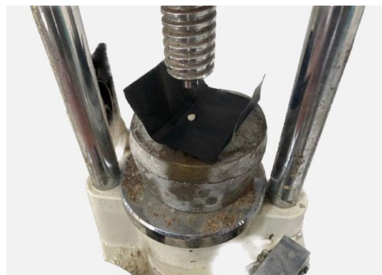
Fig 5. Disc placed in Hydraulic press
