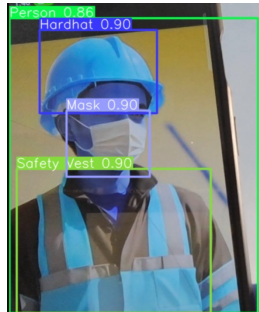
Figure 4. The person is detected with a Helmet, Mask and Safety Jacket.
