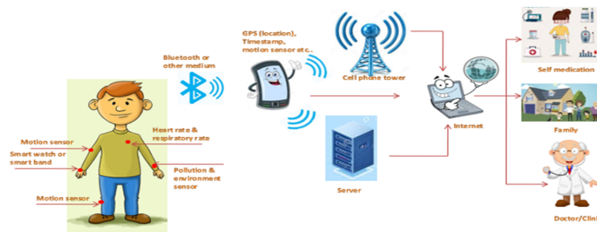
Figure 4. Schematic representation of connecting the sensors with various network sources
